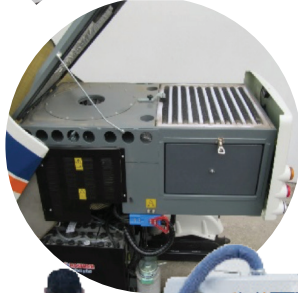
PM10 polyester filter for dust control system with electric filter shaker
