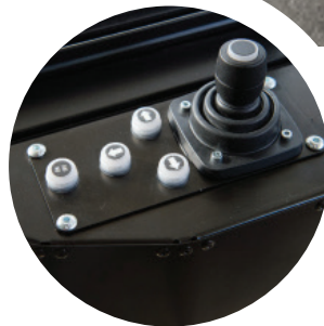
Joystick for the manual control of the front washing bar
