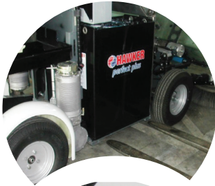
Quick battery-replacement system
