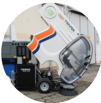
Fiberglass tilting body
