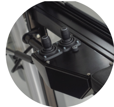
Manual and automatic independent “turn & follow” movement of brushes controlled by joystick
